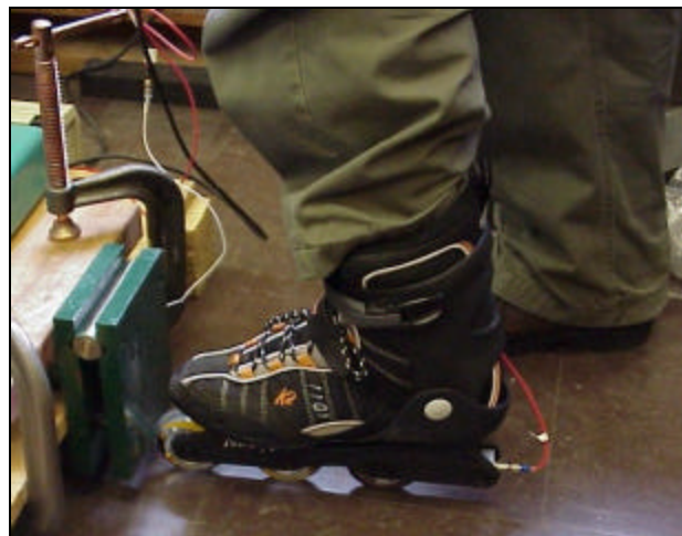
Figure 4. Experimental setup for human subject kick testing of inline skates.
