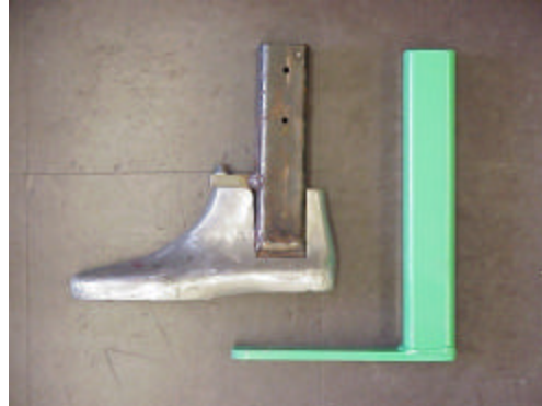
Figure 3. Comparison of prosthesis used in this study (left) and typical prosthesis used (right).
